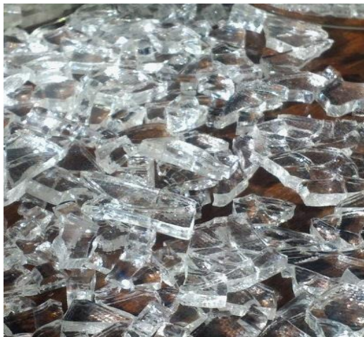
Fig. 2: Broken toughened glass
